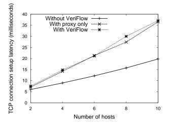
Figure 3: TCP connection setup experiment using Mininet and NOX. The verification phase of VeriFlow incurs minimal overhead compared to the proxy operations.
