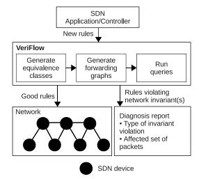
Figure 1: VeriFlow sits between the SDN applications and devices to intercept and check every rule that the network experiences.
