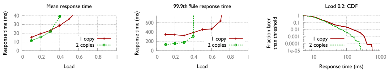
Figure 8: Cache:disk ratio 0.01 instead of 0.1. Higher variability because of the larger proportion of accesses hitting disk. Compared to Figure 5, 99.9th percentile improvement goes from 2.3 \times to 2.8 \times at 10% load, and from 2.2 \times to 2.5 \times at 20% load.
